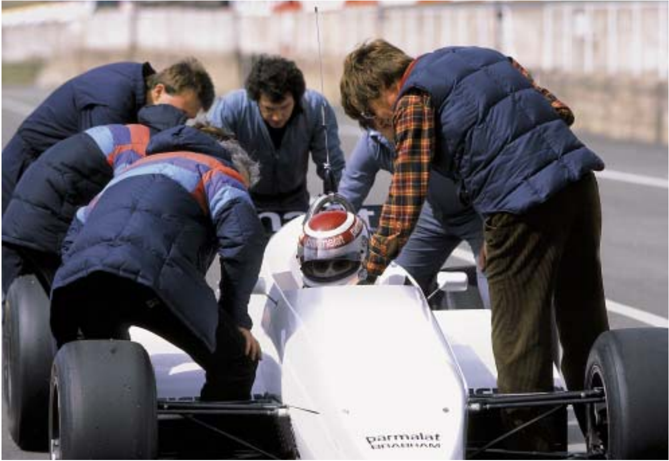
Above | The first test cars clearly displayed the long data transmission aerial.
