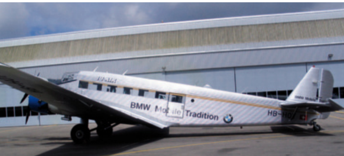
Left | A new look for the 67-year-old: the JU-52/3mg4e dating from 1939 in the livery of BMW Mobile Tradition. Beneath the blue engine cowling, the BMW 132A aero-engines with 650 hp each.
