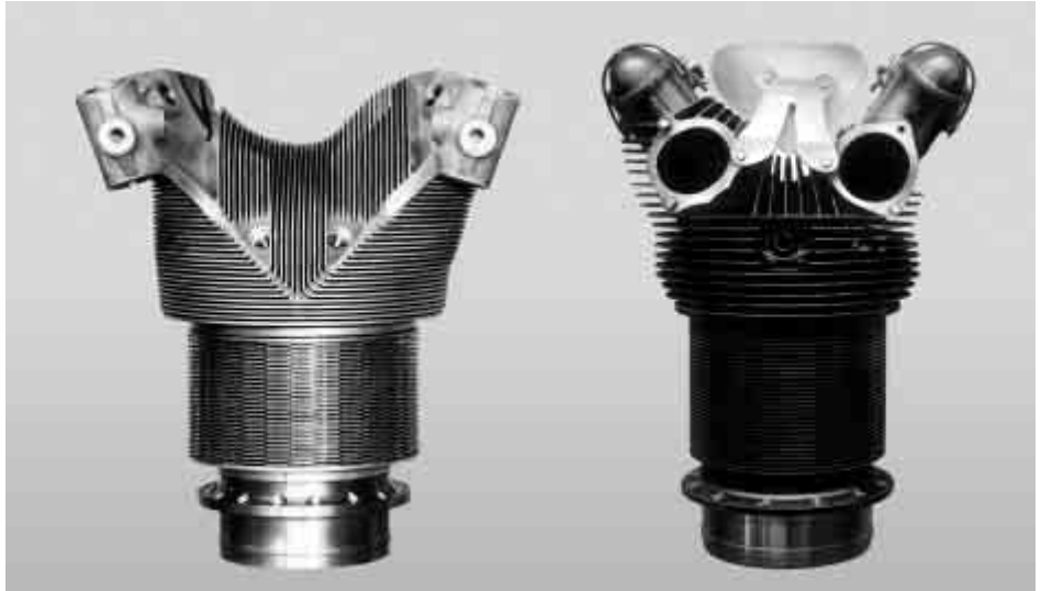
A cylinder head from the Hornet A (right) and the BMW 132 L (left). The much thinner cooling fins of the BMW 132 are clearly visible.
