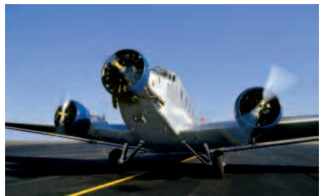
The Ju 52 from the front. Clearly visible, its blue engine covers which reduced drag and improved cooling.
