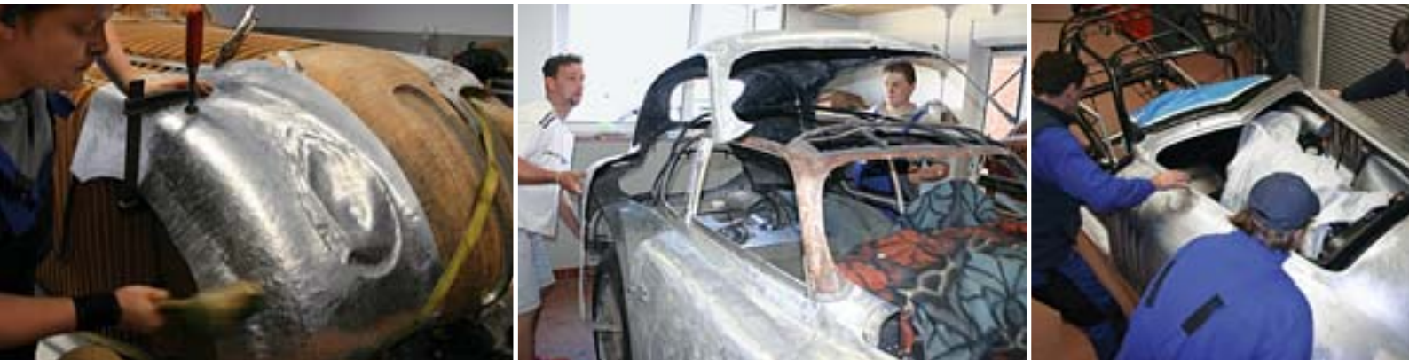
Sequence above | The fine art of bodywork construction. Sheets of aluminium are shaped for the BMW 328 Mille Miglia Coupé Touring over a wooden mould. The individual components of the body are then precisely mounted on the filigree lightweight frame in a process involving numerous steps.
